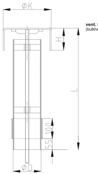
vent. bend type B (bulkhead mounted)
