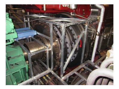
Börger is specialist in delivery of engineroom floor systems. Our delivery program comprises design, material package delivery and mounting. Depending on specyfication and class requirements floors are delivered in steel or aluminium. The floor plating can be bolted or welded and provided with hatches for e.g. valvecontrol. The floor framing consists of special galvanized system profiles.
